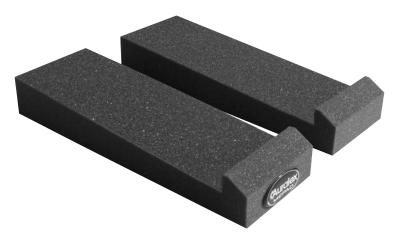
MoPADS are high-density foam products that are designed to decouple your speakers from any surface they set on in your room, whether that be a desk, shelf or speaker stands. This will "tighten" the tone of your monitors - especially at the low end - and help to reduce the amount of vibration transferred to other gear that would normally be coupled with the monitors, thus degrading your sound.
